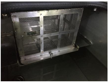
Filter screen for rinsing It's stainless steel, which can be cleaned regularly
